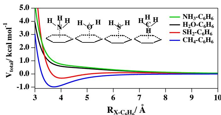
$\text{H}_2\text{O}\text{-C}_6\text{H}_6$ ,  $\text{SH}_2\text{-C}_6\text{H}_6$ ,  $\text{NH}_3\text{-C}_6\text{H}_6$ , and  $\text{CH}_4\text{-C}_6\text{H}_6$  intermolecular interaction potentials for the represented molecular approaches
