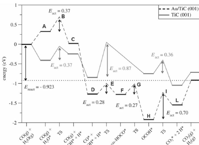
Energy derived from DFT calculations for the WGS reaction on clean TiC(001) and Au<sub>4</sub>/TiC(001). TS = transition state.
