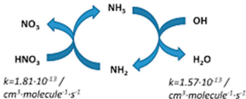
Catalytic cycle involving the oxidation of NH<sub>3</sub> by OH radical and the reaction between amidogen radical and nitric acid
