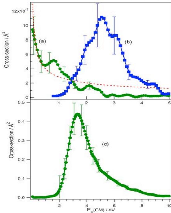
Cross-section CM energy dependences in K<sup>+</sup> + *i*-C<sub>3</sub>H<sub>7</sub>Br collisions for: (a) [K-*i*-C<sub>3</sub>H<sub>7</sub>Br]<sup>+</sup> adduct formation (●); (b) dehydrohalogenation reaction (■); (c) adduct decomposition reaction. Discontinuous line: LGS model (energies are given in the CM frame)
