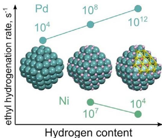
Understanding hydrogenation on transition metals: Subsurface hydrogen,  $H_{\text{sub}}$ , is shown to significantly influence the stability and the reactivity of the adsorbed hydrogen on transition metals in two different ways. Very surprisingly, density functional calculations on a representative reaction, ethyl hydrogenation, show that it is accelerated on Pd and Pt, but slowed down on Ni and Rh in the presence of  $H_{\text{sub}}$ .
