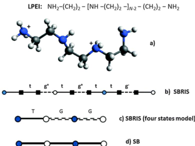
Possible ionization and the conformational state of a linear polyethylenimine (LPEI) oligomer with four amine groups. The conformation and charge distribution of the polyelectrolyte is treated at different levels.
