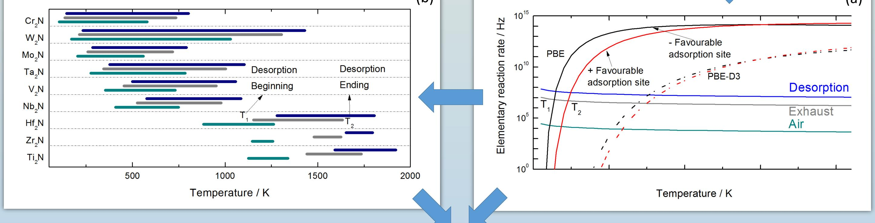
Adsorption/desorption temperature ranges (b), are obtained by the corresponding rates (a) for each material and adsorption site:
