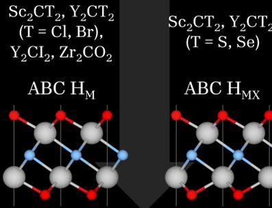
**Methods:** DFT with PBE0 hybrid functional for electronic structure and GW-BSE for optical properties.
